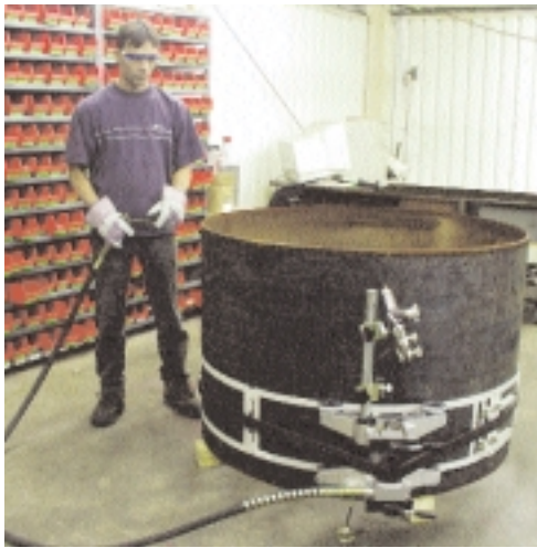
Maxi cutting on 48" / 1219mm pipe with Guide Strip and Cable Drive Assembly.
